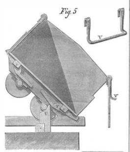
The practical miner will readily see and understand the varied advantages of this combined apparatus. From its rapidity of operation it is admiraemployed in coal yards in delivering coal, and can be used in loading or unloading ships or boats with coal, requiring the services of only one man where three are now employed.
