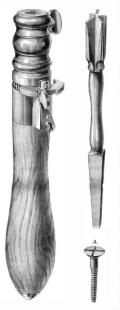
of splitting the head of the screw when the friction is great, has led to the improvement illustrated in the engraving. If the blade of the common driver does not fit exactly the slot in the screw head, the bearing of the blade is on two opposite corners of the head, the weakest part of the screw, so that not unfrequently the beveled head flies off, breaking at the slot.
