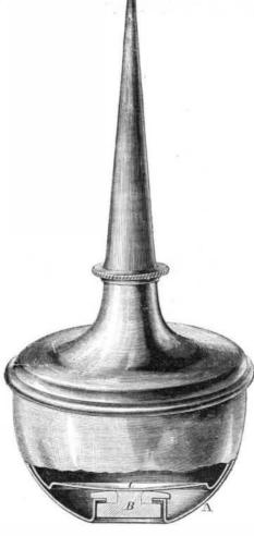
course a stove, if convenient, is the first resort in such an emergency, and the oil cup is immediately placed on it. As a consequence the bottom, which is spun in and soldered, gets leaky, with disagreeable results. Moreover, as spring bottom oil cups are usually made, the bottom is often "set" or dished by unnecessary pressure, so that in a short time it is useless for its office.
