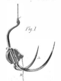
construction it is quite simple, having two tines, A, connected to a circular shank, B, which contains the tripping apparatus to discharge the load. This is simply a latch, C, so arranged that, by pulling a line, D, the latch is released and the load discharged—the parts reconnecting themselves again in the act of reloading the fork.
