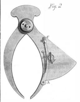
measure with great nicety. The independent leg can be fastened at any time by the thumbscrew, F, so that it is an ordinary pair of callipers. This is one of the neatest as well as most substantial tools of its class that we have seen. The implement sent here was beautifully finished; it the inventor furnishes as handsome goods to the trade he will become famous. Application for a patent pending through the Sci-
