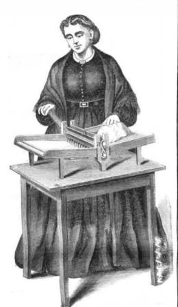
in between them; the motion is then reversed, and the same process takes place, being repeated as often as deemed necessary. All parts of this machine are easily taken out and cleaned, should dough adhere, and it may be also used for working butter.
