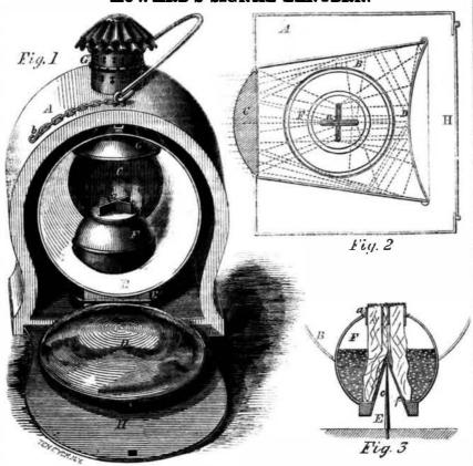
its conformation, collects the rays of light | to any of the signal lanterns now in use, far from the lamp, and throws them in a very condensed form upon the lens which sends them forth in all their intensity and brightness to illumine the darkness for a great dis-
