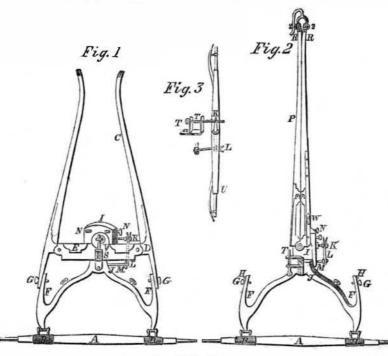
disengaged, and the horse is at once loosed from the carriage. The cross-piece, E, has a joint, V, in its center, and the bolt, K, passes through the joint, V. When the ends of the shaft at its connection, F, with the pole bar, J, are unscrewed by the screw, G, the shafts will operate and close at the joint, V, and
