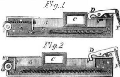
Our illustrations show it with the front plate off, that its working parts may be seen, Fig. 1 being as it would keep the belt on one pulley, and Fig. 2 as it would keep the belt on the other.
