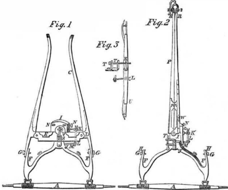
disengaged, and the horse is at once loosed from the carriage. The cross-piece, E, has a joint, V, in its center, and the bolt, K, passes through the joint, V. When the ends of the shaft at its connection, F, with the pole bar, J, are unscrewed by the screw, G, the shafts will operate and close at the joint, V, and
