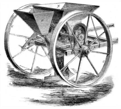
phery is in contact with the periphery of the planting wheel, so as to enable the two to turn together, and immediately above the portions of these wheels next each other is secured a hopper, N, on the front part of which is secured a knife, whose cutting edge is brought in tangential relation to the periphery of the planting wheel or roller, G, so as to cut off any portion of the seed potatoes in the openings or indentations of the same, and thereby bring them to one uniform size.
