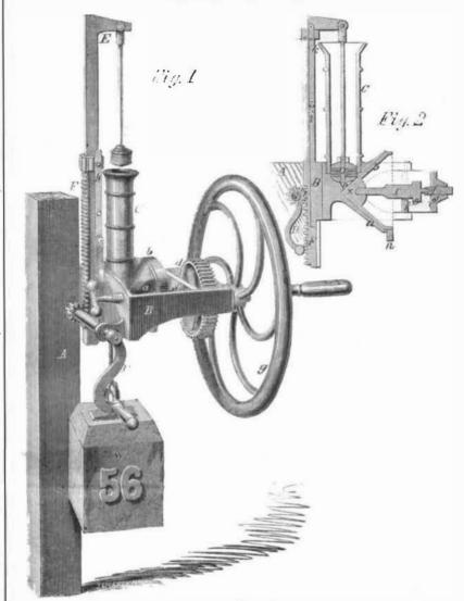
Although paint can be ground very finely | during the process of grinding. The muller, and well with a muller and stone, yet the operation is very tedious and slow, and it has been found advisable in this, as in every other branch of manufacture, to introduce machinery. Our engravings illustrate a mill for grinding paint with expedition and evenness. Fig. 1 is a perspective view of the mill, and Fig. 2 a vertical section of the same.
