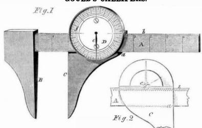
parts of an inch, with relation to the inches on A, as may be desirable, so that, as C is moved the toothed wheel, c, rotates, carrying with it the pointer, e, by whose means the exact size of the object or the distance apart is dated April 12, 1859.
