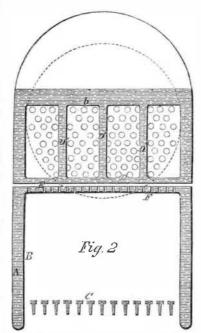
the superior density of the fluid, and the invention in practice supplies the air in the very heart of the furnace and diffuses the streams uniformly throughout the whole area so as to fill the space with an intensely hot flame.
