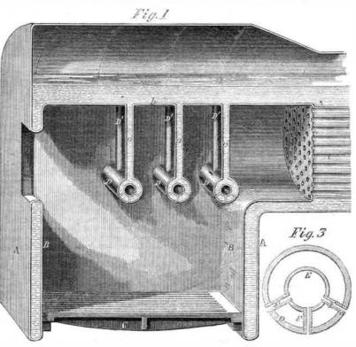
flow into the furnace. The annular space between D and E communicates with the water of the boiler, which circulates actively through, coming in from each side and ascending, mingled with steam, through the vartical pipes, D'.
