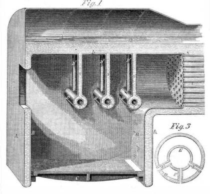
flow into the furnace. The annular space between D and E communicates with the water of the boiler, which circulates actively through, coming in from each side and ascending, mingled with steam, through the vertical pipes, D'.
