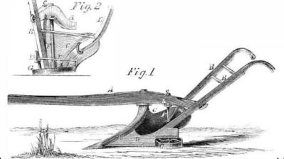
As the plow gudes through the earth, the of the land side and mold-board; in the inmeasure, and also a means supplied of regulating the plow, so that it will form furrows of greater or less depth as may be required.
