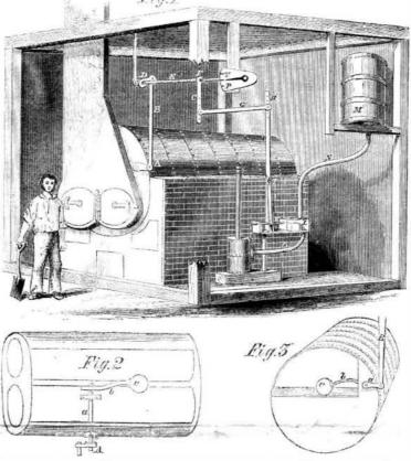
There is little doubt that a great number of the explosions which take place upon our western river steamboats, are caused by an inefficient supply of water to the boilers, and the boiler becoming red-hot, a great quantity of water is thrown into the spheroidal state, and the moment the boiler cools, either from the fire lowering or the introduction of fresh fuel, the water bursts into steam and causes the horrible accidents that are so often detailed in the newspapers.
