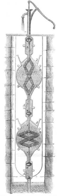
water from the well is drawn up. When B is depressed, it passes through the water in A by its clack valve being opened, and compressing the rods, b C, elevates the piston, B'. thus bringing up more water, and at the same time the opening of the cross-rods and links, b' and C', depresses the piston, B," and the weight of water closes a.
