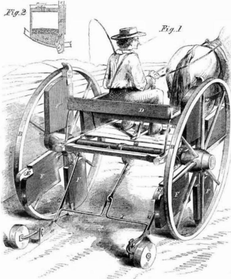
or fall in register with the recesses, e, in the bars, E, and the seed will be discharged into the holes in the earth made to receive it, by the projecting or outer ends of bars, E. The recesses, f, as the seed is discharged from the recesses, e, are filling with seed to be discharged at the succeeding revolution of the wheels. The shares, H, cover the seed; they may be elevated at any time by operating the front of the lever, which may be retained by any suitable catch or device.
