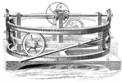
S, give motion through another one to the belt wheel, K, by which the power can be conveyed to any machine desired. By varying the proportions of these wheels, any desired relation between the velocity of the horse and | Park-place, New York.
