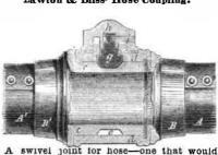
admit of turning, and that could be easily put together-has long been wanted. Here it is. It is the invention of R. B. Lawton and W. H. Bliss, of Newport, R. I., and was patented Feb. 22, 1859. Our illustration fully shows the invention, the coupling being seen in section.
