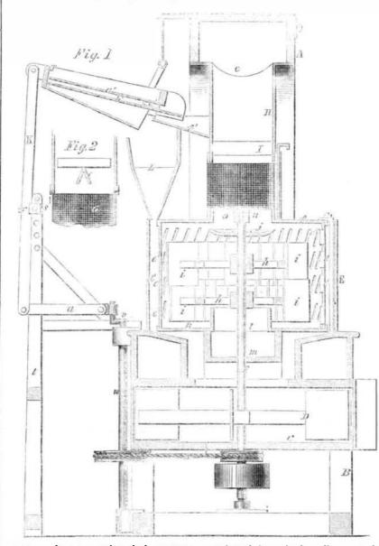
grain passes down a spout into the lower part of A, where it is subjected to a second blast, and falls away in a perfectly clean state. All light grain is carried by the blast to one discharge spout and the heavier into another, the
