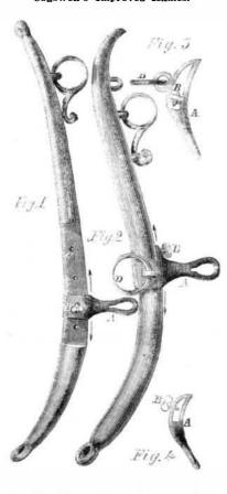
The shafts of different vehicles vary in height, and horses are by no means all of the same size. Now it is important for the horse when drawing a vehicle, that the line of draft from the traces should always come in the same place on the horse, which cannot be the case when the eye is rigidly attached to the hame, for if it be properly set for one horse or vehicle, it is obvious that it must be far from correct for another horse or vehicle.
