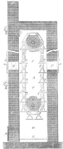
A is an elongated hollow, vertical column, square or about so in horizontal section, and covered at top, the lower part of the space within the column being provided with a grate, B, extending across it. An opening, C, made through the front wall of the hollow column is furnished with a door, D, and constitutes the mouth of the furnace, all the space above being what may be termed the baking
