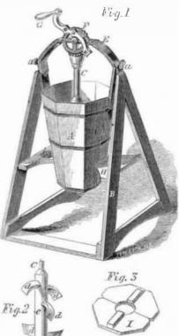
working shaft (seen better in Fig. 2), having on the end that is placed in the churn an enlargement, c, from which project a series of pivots, a, on the frame, B. The churn can dashers, d, of the shape or form shown in the
