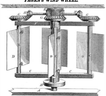
No wheels whose sails are arranged vertically will operate without they have some arrangement by which they can be made to present a full face to the wind on the one side, and their edge to the wind on the other, so that the full force of the wind may be exerted sail may offer very little resistance on the
