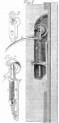
This is an invention for keeping the window in any position in the sash, and is very simple and efficient. Fig. 1 is a view of the window-frame with it attached, Fig. 2 shows the fastening detached, and Fig. 3 a view of the center casting.
