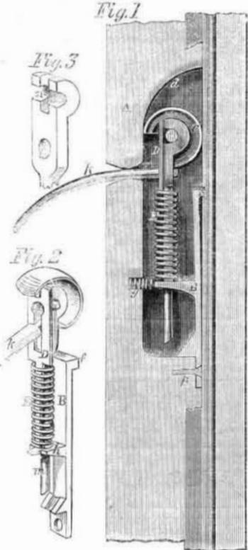
This is an invention for keeping the window in any position in the sash, and is very simple and efficient. Fig. 1 is a view of the window-frame with it attached, Fig. 2 shows the fastening detached, and Fig. 3 a view of the center casting.
