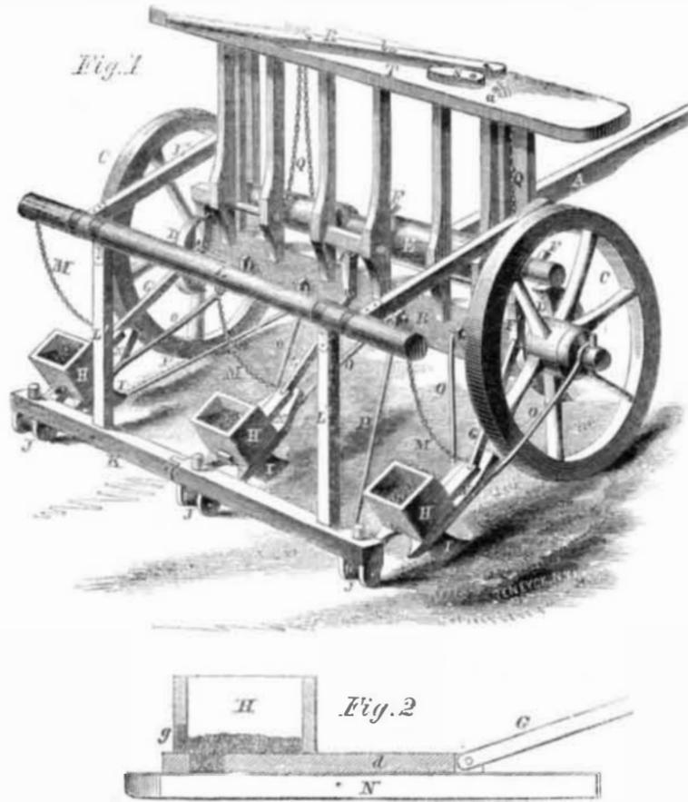
being held in proper position by the dog, or catch, S, the weighted bar is kept out of the way of the cams, D. A seed slide provided with a cut-off as well as well as slide may also be applied if desired, but the form we have engraved is, as we said before, cheap and sim-
