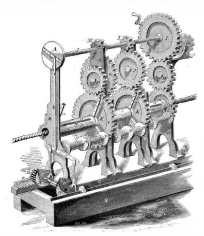
to the center of A, the stroke of the rocker, 6, on guides, e, on the ways, Q. The three sepaand bars, 5, 5, will be lengthened or shortened and the number of ratchet teeth on the wheel, B, taken by the ratchets, C, will be correspondingly altered, and the progress of the driving cog, D, upon the stationary rack accelerated or retarded. The machine moves by addressing him as above.
