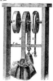
A three-ply belt of the same diameter, length, and thickness as the leather one, was chosen. and being loaded with 32 pounds to keep it "taut," weights were added, as in the former instance, and the result was as follows :-
