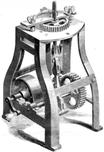
table itself, as well as by a permanent clamp, J, that is held down on the wheel by the screws, d, and nuts, c. The saw, G, works up and down in a slot in J, and it is pressed against the inner periphery, or provided with further particulars upon being addressed as the requisite feed by a spring, a, that can be above.
