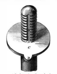
the nut to prevent the latter from becoming loosened. The object is to prevent the loosening or loss of nuts or barrs where exposed to jar or tremulous motion, and in many places will answer a very desirable purpose. Patented May 29, 1866. through the Scientific American Patent Agency, by G. G. Hickman, Coatesville, Pa., to whom address for further information.
