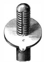
the nut to prevent the latter from becoming loosened. The object is to prevent the loosening or loss of nuts or burrs where exposed to jar or tremulous motion, and in many places will answer a very desirable purpose. Patented May 29, 1866, through the Scientific American Patent Agency, by G. G. Hickman, Coatesville, Pa., to whom address for further information.
