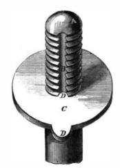
the nut to prevent the latter from becoming loosened. The object is to prevent the loosening or loss of nuts or burns where exposed to jar or tremulous motion, and in many places will answer a very desirable purpose. Patented May 29, 1866, through the Scientific American Patent Agency, by G. G. Hickman, Coatesville, Pa., to whom address for further information.
