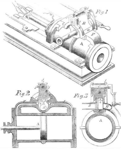
engine, the valve is made stationary, and with its face concave to fit a seat on the cylinder in the form of an arc generated from the axis of oscillation of the cylinder, and the steam and exhaust pipes are attached to the valve instead of to the cylinder; the steam pipe being attached to communicate with the cavity, h, and the exhaust pipe with above.
