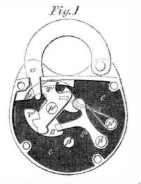
This lock causes the bolt to be shot ing over the pin, p', and supporting B. The through the shackle by the action of the other projection is a stud, which affords a shackle itself, but it cannot be unlocked except by the key from without. Our engravings fully illustrate the invention, which was patented January 26, 1858-Fig. 1 showing the shackle and bolt in a locked position, and Fig. 2 in an unlocked one.
