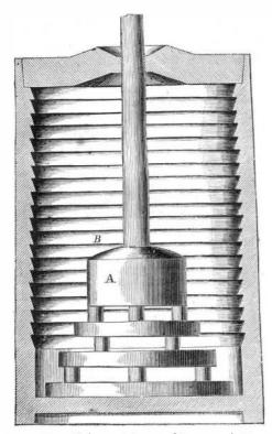
to and fro as it is dashed up and down in the cream. In this way air is carried down with it at each stroke and the cream forcibly ejected through the holes in the dasher against the corrugated interior of the
