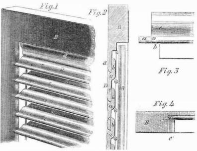
the weather. This weather-strip is seen at C, Fig. 4, and the slats are operated by an inside piece, A; they turn upon a pivot, a, which is cut with the slat and forms part of it. The invention consists in hollowing out the back, b, so that the front, c, of the slat above it will overlap, and also providing the strip, C, against which the slats fall flush, and so prevent the ingress of rain and bad weather generally.
