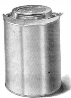
These engravings represent an improved can for the purpose, which is admirably adapted for its object. The can has a tin cover, A, fitting over a projecting rim on the body of it; said rum having a rubber joint or gasket, B, let into a recess so that it cannot slip off. When the fruit is in and properly scalded, the cap is pushed down and immediately seals it up from contact with the air.
