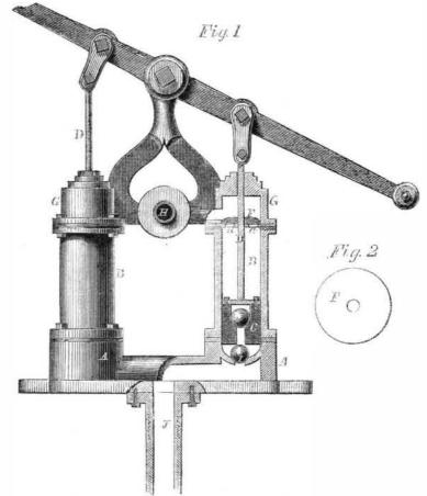
ber in G, and so to H, as in other force | next upward stroke. There being two cylinpumps, the valve in the piston being closed, the water follows it through the valve, I. When the piston descends, the valve, F, closes and retains the water above it, and I
