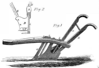
ordinary surface plow available when necessary as a sub-soil one. To effect this, a supplemental land-side and a coulter attached to the plow are used. Fig. 1 is a side, and Fig. 2 a front view of the improvement.
