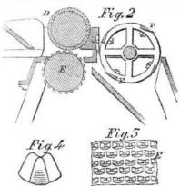
Between these the feed rollers, D E, are placed. The lower one, of which E has upon its surface a number of teeth shaped like the molar teeth of animals, running in a zig-zag
