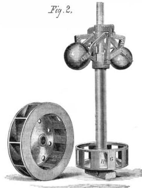
the end of a bell crank, D. The other end of the same connects with a collar on a cast-iron sleeve, E, fitting over the main shaft, and the governor levers also connect with it through the medium of a bolt, F. The sleeve, E, connects at the bottom of a regulator valve, G, Fig. 2.
