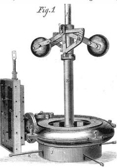
the duty to be performed at the moment, otherwise irregularities are manifest. This must be done by the wheel itself, automatically. It cannot be done by hand, for no human intelligence could foresee the precise moment when a machine was about to put on or off in the mill.
