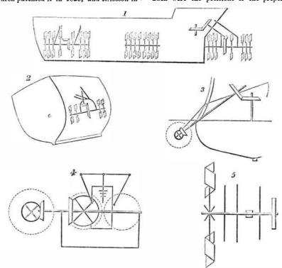
when in use: but it was soon found needful to have a power of altering the position, so as to hoist it out of the way. For this purpose, Bernouilli (1752) put hinges on the rods supporting his side propellers, and detached the propeller from the shaft at the stern. Others left the propeller free to revolve as the vessel sailed. Slaughter (1849) helped it to do so view of a section of the propeller.
