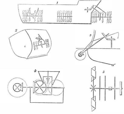
when in use : but it was soon found needful to have a power of altering the position, so as to hoist it out of the way. For this purpose, Bernouilli (1752) put hinges on the rods supporting his side propellers, and detached the propeller from the shaft at the stern. Others left the propeller free to revolve as the vessel sailed. Slaughter (1849) helped it to do so view of a section of the propeller.
