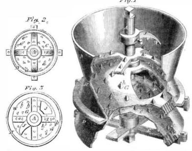
bark will be sufficiently reduced to pass down between the shell, C, and case, D, and escape from between the fine teeth, e b, thereof, in a properly ground state.
