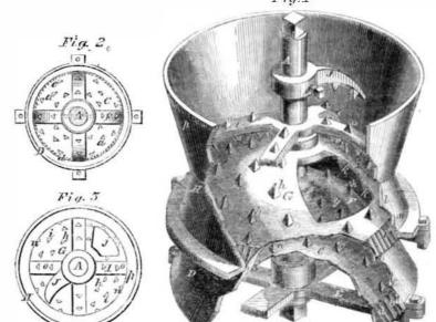
bark will be sufficiently reduced to pass down between the shell, C, and case, D, and escape from between the fine teeth, e b, thereof, in a properly ground state.
