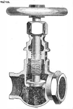
Unless such valves are again accurately fitted to their seats by regrinding, the steam soon cuts into them deep grooves and channels. The trouble attending this operation, in ordinary globe valves is so great that it is generally neglected until great loss is incurred by waste of steam, and sometimes se rious incidental damages.
