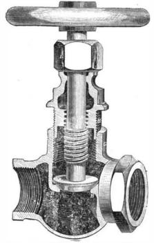
Unless such valves are again accurately fitted to their seats by regricding, the steam soon cuts in o them deep grooves and channels. The trouble attending this operation, in ordinary globe valves is so great that it is generally neglected until great loss is incurred by waste of steam, and sometimes serious incidental damages.
