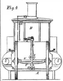
pump making 240 revolutions and discharging 1,100 gallons of water per minute, and the boiler supplying abundance of steam at this speed, with a pressure of 150 pounds to the inch. This performance is believed to be unprecedented in the history of hydraulic machinery of a portable kind, whether for steam fire-engine purposes or any other.
