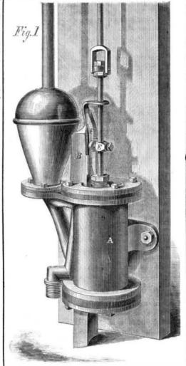
In the perspective view, Fig. 1, one form of this pump is shown, and also the means used to operate the piston; the latter, be it understood, turns slightly in the coupling, but is fast on its rod, so that the flanges can open or close the water ports. It may be
