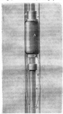
threat cut on the main tubing. E E, are elliptic springs, dove-tailed or otherwise fastened to the sides of the loose nut D, and partially clasping the tubing at F, also pressing the walls of the well at G, thereby holding the loose nut firmly and preventing its rotation.
