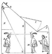
interior of the box is divided centrally by the partition, K K, made of a good, clear, and even-surfaced piece of thin patent plate glass, kept in its place within two side grooves. The box is thereby divided into two separate chambers or compartments, L M, the former, L, having a ceiling or screen, N, to exclude any object therein from the direct view of the spectator, as shown by the line, a b.
